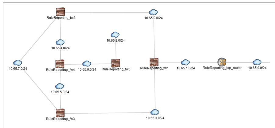
Figure 1. Juniper Secure Analytics Risk Manager topology viewer enables users to see network devices and relationships, including subnets and links.
